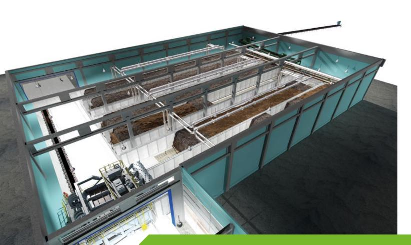
The BioFIX turning machine starts from the discharge traversing system and moves to the waste material on the top of bin walls via rails.
