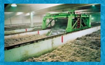
Fully automated, dynamic rotting process Actively ventilated rotting lines High quality exhaust air treatment
