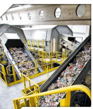
The later installation of another NIR separator can optionally be prepared to further improve the product quality. This optional NIR separator would then be operated negatively, i.e. interfering material would be discharged by a blow of compressed-air. The LDPE product thus obtained is conveyed to the sorting cabin and is sorted there for interfering material on the sorting belt. The reversible belt conveys the overflow of the sorting belt to the bunker or the opposite bunker.
